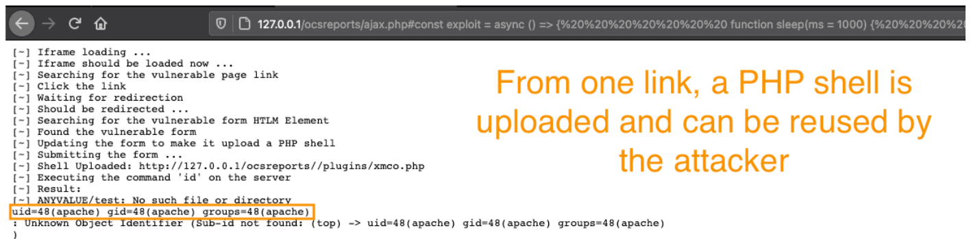
Capture 1.4: Exploiting the remote code execution vulnerability from the XSS
